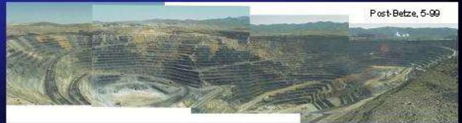
**The open pit at Post-Betze – large-tonnage, open-pittable deposits – ~40 Moz of gold at a grade of ~5 g/t.**
